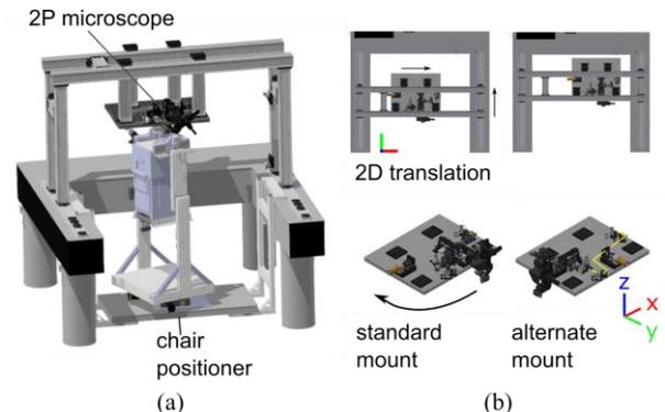
Figure 1: (a) Model of microscope and chair positioner assembly. (b) (top inset) Translation range of the microscope table (top), and rotation range of the detection arm. (bottom inset) Standard and alternate mounting positions of the microscope.
