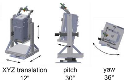
Figure 2: Motorized axes of the chair positioner.
